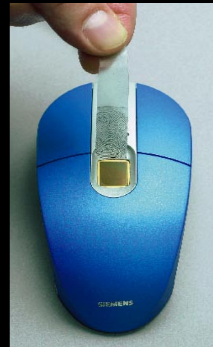
graphite powder on adhesive tape
